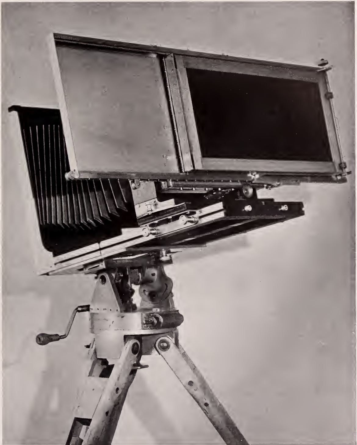
Three-Color Camera, repeating-back type, constructed by Mr. Doolittle. With it three 5x7 color corrected negatives may be made in an interval of 3 seconds
